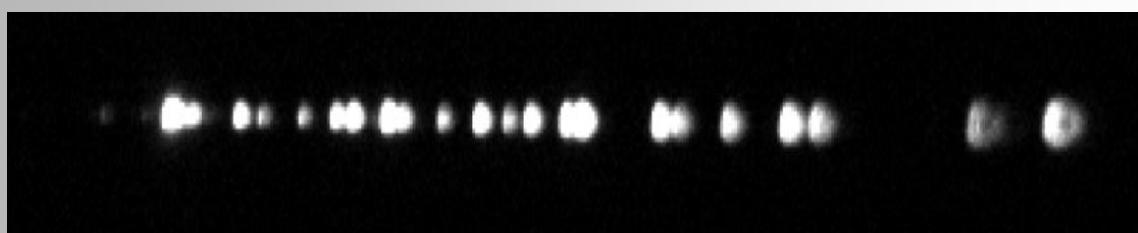
**Fig. 9:** Enlarged imaged of the neon emission lines from the slitless spectroscope.
