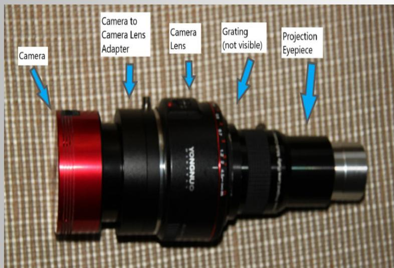
**Fig. 6:** Here is the full slitless spectroscope. It weights 1lb 5oz (600 grams). This is a lot of weight to hang off a small telescope.
