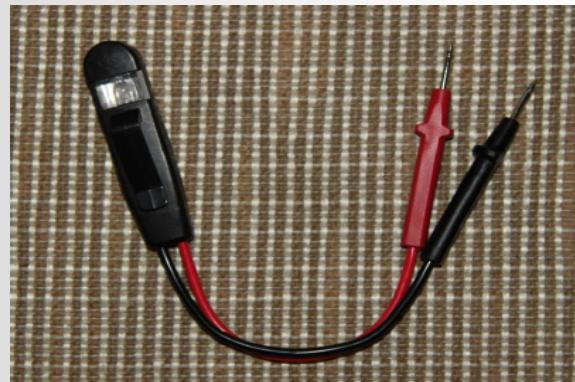
**Fig. 2:** The Neon light source: these neon test lamps are used to determine the presence of electricity. They glow when the voltage is over 90v. They are common and can be found in most hardware stores for \$3.
