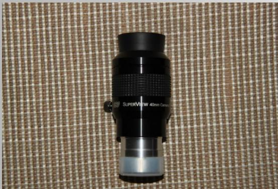
**Fig. 5:** The Collimating Lens;The top of this 1.25" Plossl eyepiece has a T / T2 male thread that can be exposed by unscrewing an eye guard. I can connect this eyepiece to the AD-T2 DSLR adapter on the lens.
